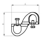
**Function:** Can be used for four direction pipe fixation. Suitable for fixing pipe  $\leq$  DN200
